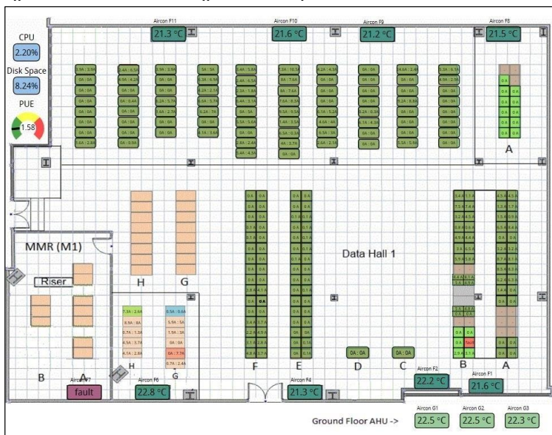
Fig 1. HTML5 Dashboard showing Datahall Floorplan
